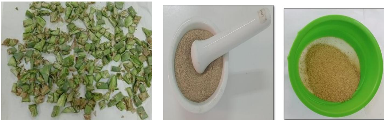
Fig. 3 Cactus powder preparation steps.
